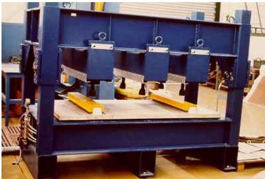
Figure 2. Photo of sandwich panel on test bed.
