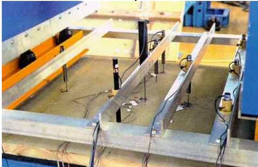
Figure 9. Photo showing displacement transducer arrangement
