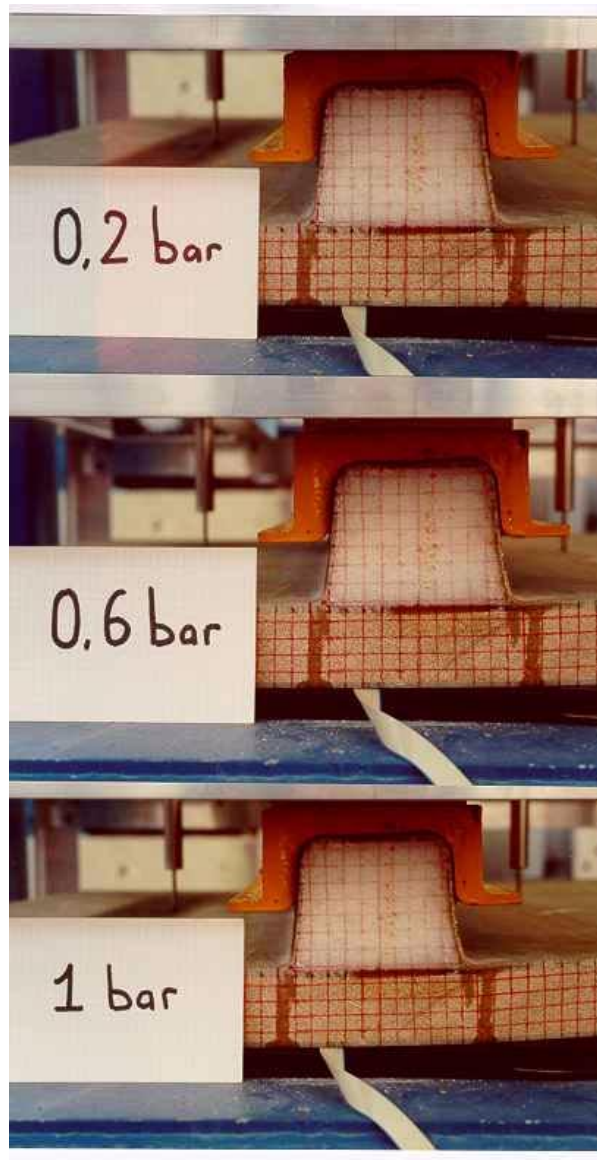
Figure 13. Stiffener end movement during loading.
